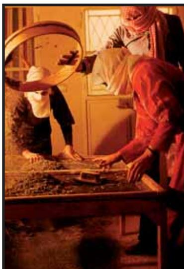
Initial screening process, the window screen used is metal, this process removes all stems, twigs,
