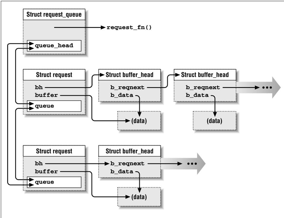
Figure 12-2. Buffers in the I/O Request Queue
