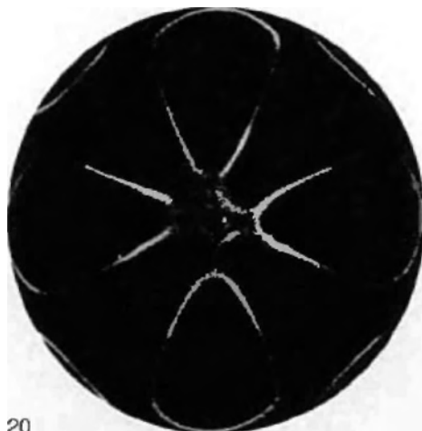
20 Sonorous figure on a circular plate. Diameter 16 cm, frequency 1060 cps. The nodal lines are made visible by sand.
