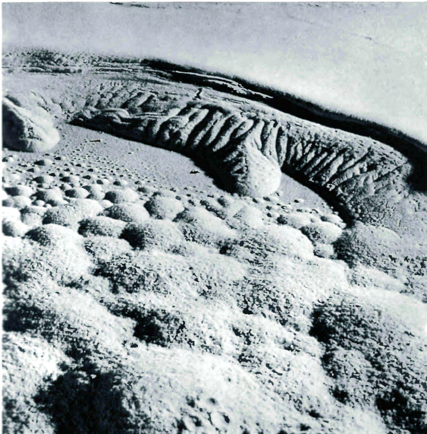
92 This landscape of lycopodium powder under the influence of vibration is a synoptic view in which the various phenomena can be recognized in all their diversity. Everything must be imagined as circulating, moving, pulsating etc. and all this is caused by the vibrations of a tone which can be heard the whole time the experiment is in progress.
